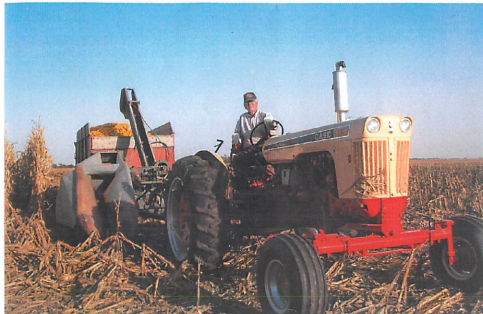
1961 CASE 730 TRACTOR, ONE ROW NEW IDEA EAR CORN PICKER STANHOIST BARGE WAGON
